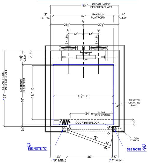
STANDARD ELEVATOR SHAFT PLAN VIEW
